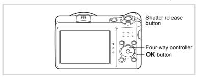
Press the four-way controller (▼) in **□** mode.
